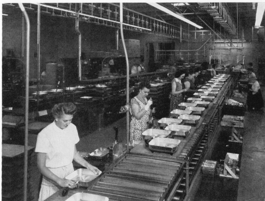
Automatic fry-pans are individually calibrated for proper temperature setting. They are then cooled on a conveyor system which (above) moves above the assembly line and crisscrosses in the rear of the photo.
