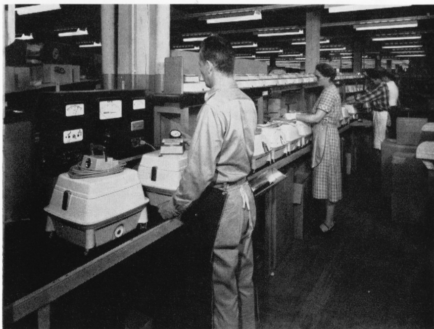
The newest item added to our Hamilton Beach line is the Model 35 Canister Cleaner. Above, each cleaner is individually tested for suction after the paper disposal bag is installed at the end of the production line.
